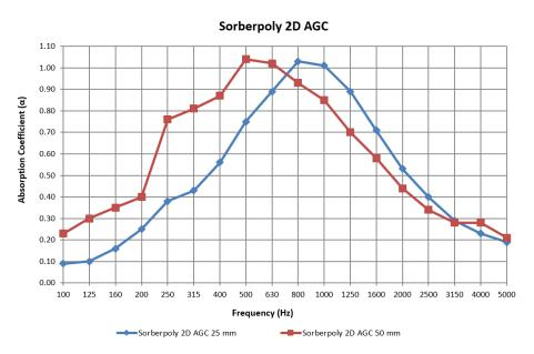
Tested to ISO 354:2003 at University of Canterbury, New Zealand | Report Numbers: 303 & 304 Acoustic results based on 32 kg/m³ density material
